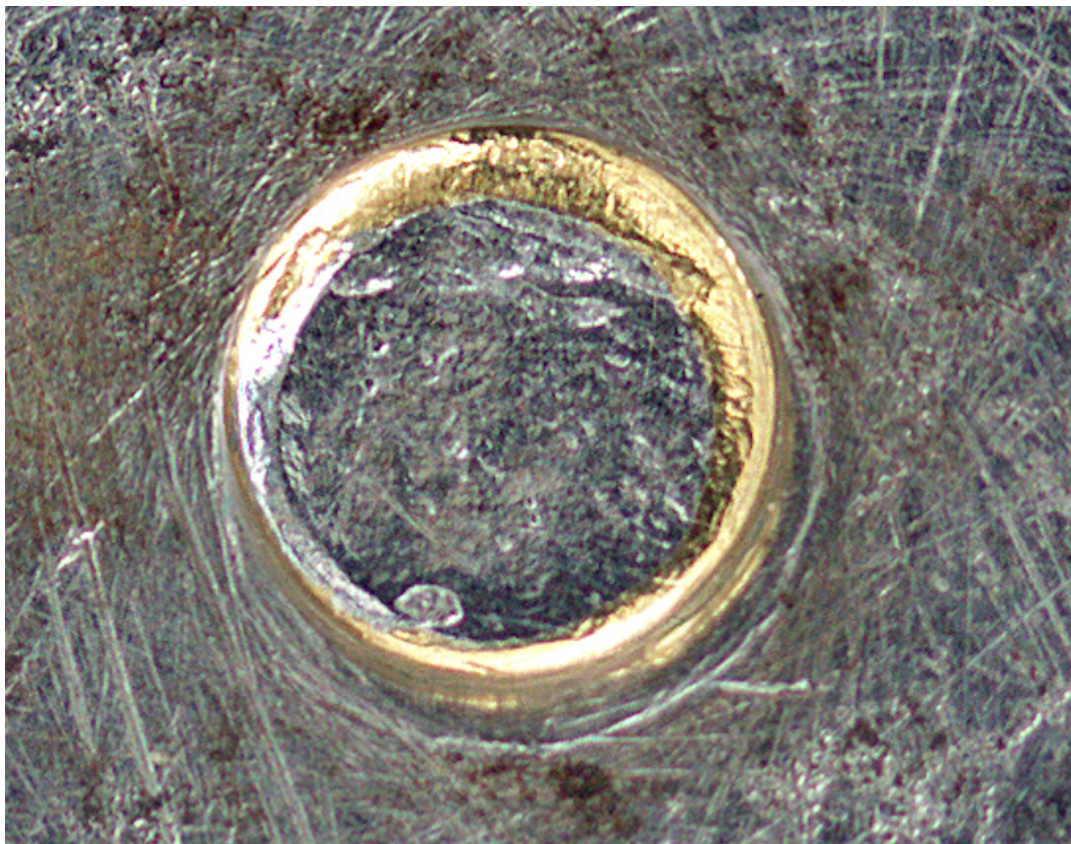
Illustration: Lined wheel axle on the hour wheel
