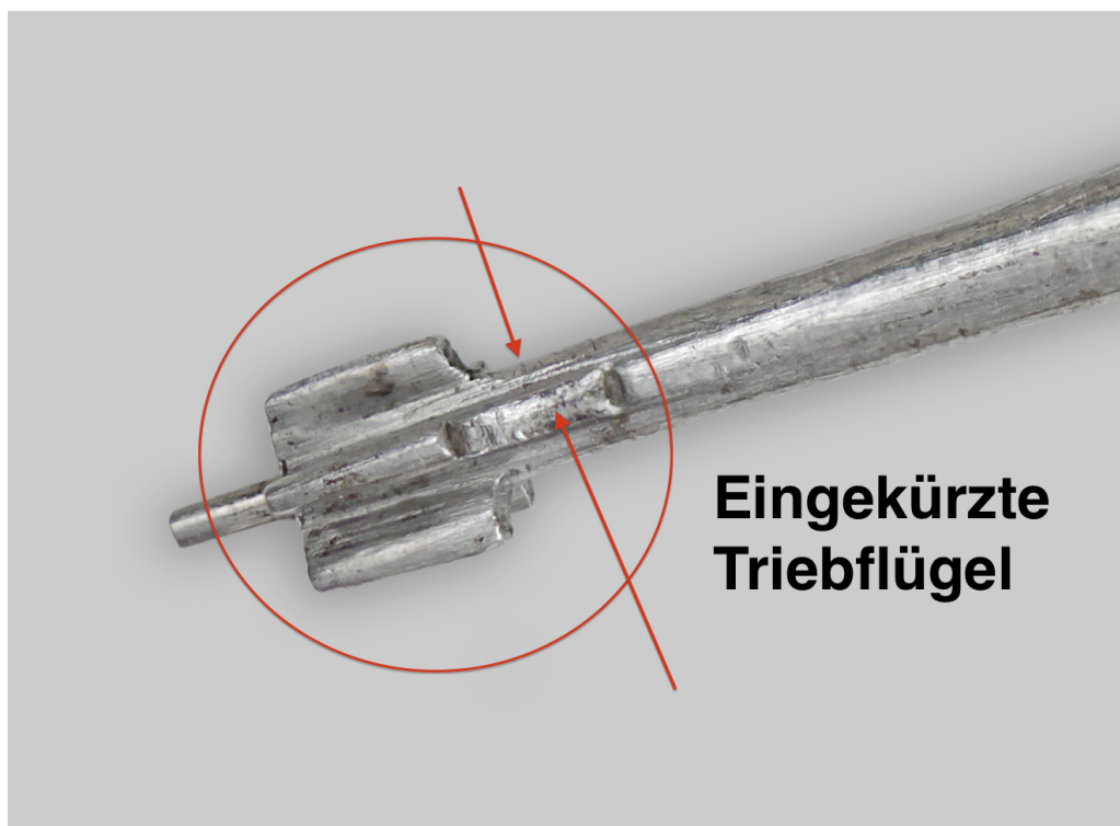
Illustration: Shortened arbor on the crown wheel
